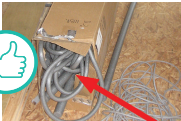
BACKER ROD FOR SEALING AROUND WINDOW
