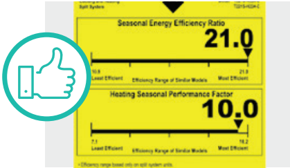
HSPF2 MEETS THE FEDERAL MINIMUM HSPF2 PER SPECIFICATION Courtesy of ENERGY STAR, U.S. Environmental Protection Agency
