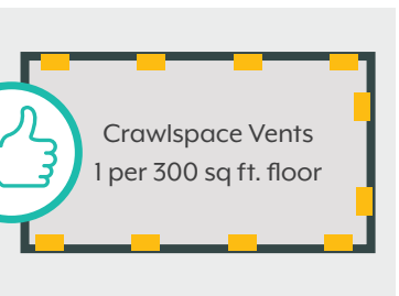
VENTED TO MINIMUM AMOUNT AND WELL DISTRIBUTED
