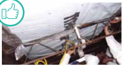
Repaired and supported belly material. Courtesy of Pennsylvania College of Technology
